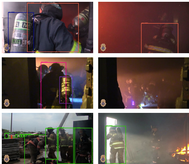
Fig. 3: Difference in performance when the model detects objects in normal conditions (left) versus smoke-filled and low-light conditions (right) for 3 videos (3 rows).
