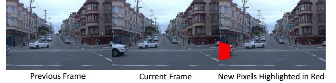
Fig. 7. An example of new pixels in the current frame highlighted in red.
