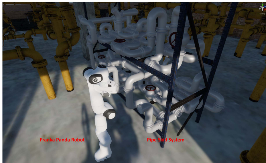
Fig. 3. The pipe skid system and Franka Panda robot in the virtual environment.
