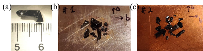
Extended Data Fig. 1 | Pictures of the \text{UTe}_2 single crystals used in the INS experiment. a , A typical piece of \text{UTe}_2 single crystal of 10 mm by 3 mm by 3 mm in size. The direction of the longest edge is the intersection of [1, 1, 0] plane and [0, 0, 1] plane. b, c , 27 pieces of \text{UTe}_2 single crystals co-aligned on two oxygen-free Cu sample plates. The total mass is 0.9 grams.
