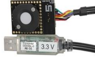
Fig. 3. Photograph of the spectral kit, AS7341 Sensor.
