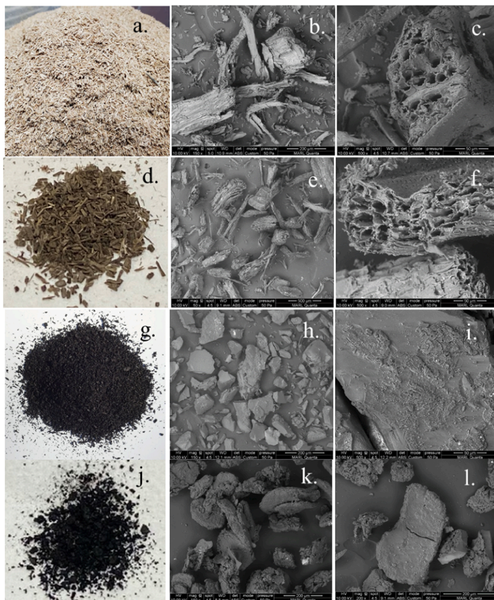
Fig. 6. SEM results. a-c. red oak; d-f. red oak alone converted in 280 °C GVL for 40 min; g-i. the solid recovered by co-converting a 1:1 ratio of red oak and PVC; j-l. the solid recovered by co-converting a 2:3 ratio of red oak and PVC. In g-l, the solvent temperature is 280 °C and the reaction time is 20 min. (For interpretation of the references to color in this figure legend, the reader is referred to the web version of this article.)
