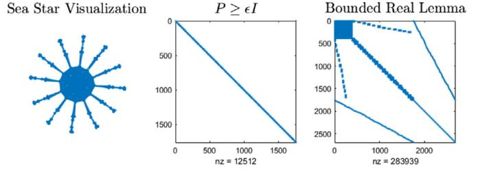
**Fig. 6.** Sea Star topology and LMI constraint sparsity.
