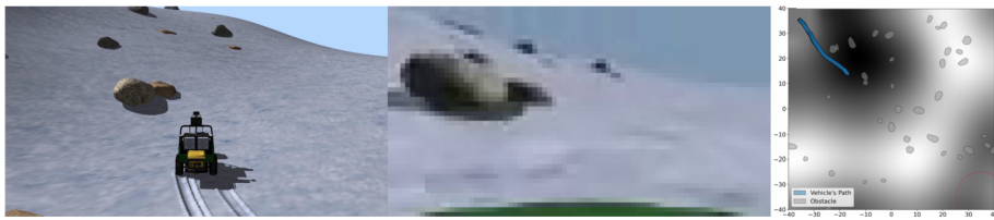
Fig. 4 Snapshot of a scenario used for testing. Left: third-person perspective of the vehicle; center: image from the camera's view at the resolution used in the training 80 \times 45 pixels; right: the current progress of the vehicle amount the hills and obstacles corresponding to the images on the left
