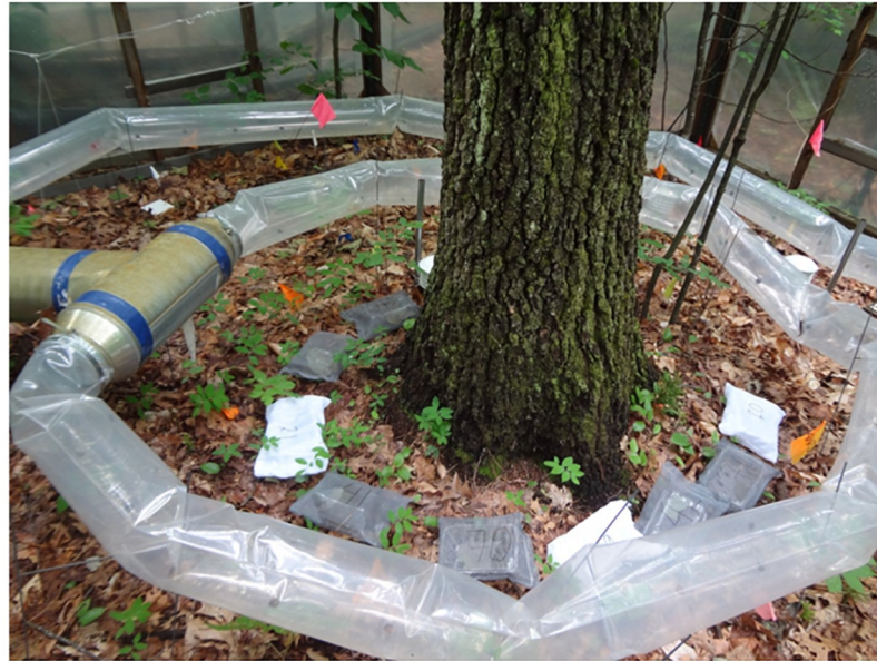
Fig 1. Litterbags placed in the Harvard Forest warming chambers. Different mesh sizes were used to control the size of the invertebrate community accessing the bags ('invertebrate exclusion treatments').
