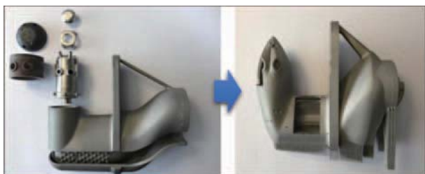
Fig. 6 GT26 lance injector demonstrating assembly reduction.
