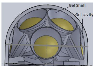
**Figure 2.** Plastic ‘gel shells’, filled with liquid gel in *in situ* method.
