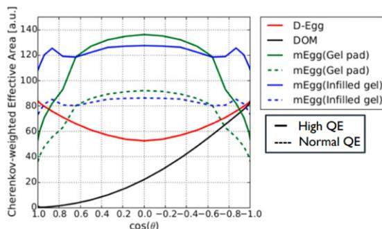
**Figure 6.** Using a model with  $14 \times 4''$  PMTs in the D-Egg vessel (mEgg), gel pad performance is compared to the DEgg and Gen1 DOM as baselines. A comparison is also made to an mEgg with a gel-filled interior (infilled gel).
