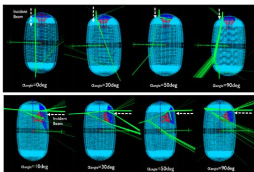
**Figure 5.** GEANT4 simulations of the response of the PMT-and-pad assembly. Photons incident outside the rim of the PMT photocathode are captured via total internal reflection off conical pad walls. The parameter  $\alpha_{\text{angle}}$  denotes the angle between the pad wall and the normal to the pad axis.
