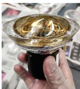
**Figure 3.** A gel pad coupled to a PMT.
