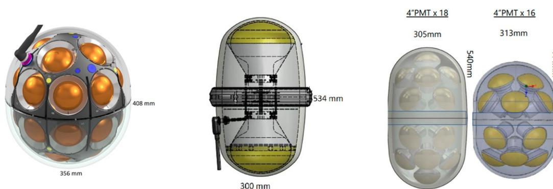
**Figure 1.** Left: the multi-PMT Digital Optical Module (mDOM). Middle: The dual-PMT Optical Module (DEgg). Right: the two LOM designs.
