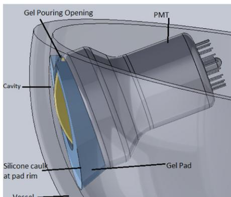
**Figure 4.** The cavity seal method.
