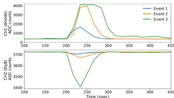
**Figure 9.** A sample event readout. Event 3 saturates the anode readout on ch. 1, but the readout on ch. 2, from dynode 8, retains event information.
