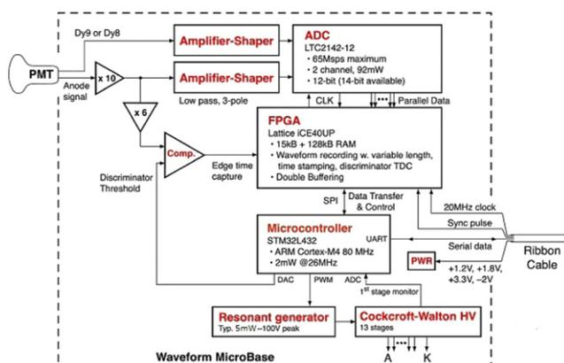
**Figure 8.** A block diagram of the Waveform MicroBase.
