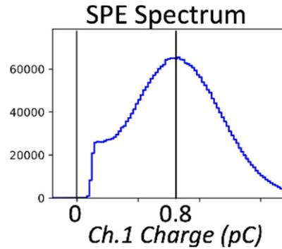
**Figure 10.** The measured charge distribution for single photoelectrons at a gain of  $5 \times 10^6$ .
