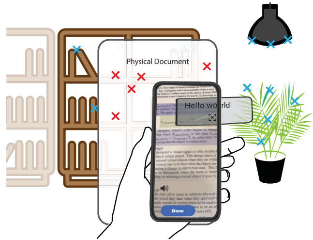
Figure 8: When the document is fully in view, it will be tracked by the image tracking algorithm (marked with a red cross). When users view annotations on the edge of the document, the system switches to SLAM tracking (marked with a blue cross)
