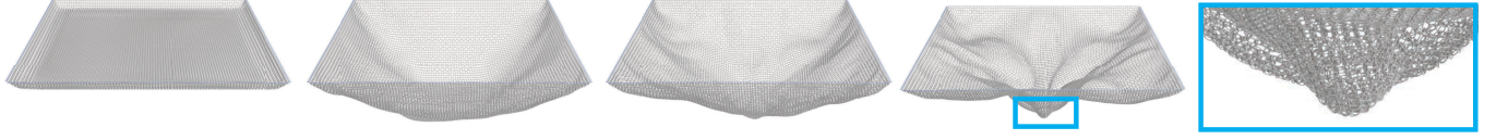
Fig. 15. Huge chain net. When the body count increases, the disadvantage of using redundant DOFs in the simulation may become more obvious. Following this thought, we up scale the chain net to 27,645 bodies. In this stress test, A-IPC takes about 5 min to simulate one frame on average. The entire simulation takes about five days with A-IPC. We are never able to finish this test with rigid-IPC. Based on our observation, A-IPC is at least 2,000 \times faster than rigid-IPC. This means it will need several years for rigid-IPC to finish this experiment.
