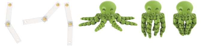
Fig. 13. Constrained simulation. Prescribing rotation freedom in ABD is convenient. We visualize the generalized coordinate as a virtual tetrahedron, and most rotational constraints are linearized. We show two examples of such simulation in this figure. Both pendulum and octopus tentacles are made of multiple bodies connected via hinge joints. ABD remains significantly faster than rigid-IPC: ABD achieves a 371× speedup for the pendulum and a 28× speedup for the octopus.
