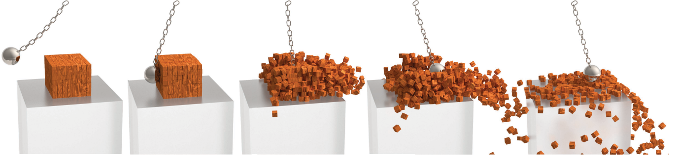
Fig. 3. Wrecking ball. A metal ball linked to a chain of rigid rings hits a stack of 560 wooden blocks. There are in total 575 bodies including the ball, rings on the chain, and blocks in this example. ABD and rigid-IPC yield nearly identical simulation results but ABD is 124× faster than rigid-IPC (both on CPU). The time step is \Delta = 1/100 sec. We also tested ABD using \Delta = 1/50 sec and \Delta = 1/25 sec respectively. The results are similar – all are free of inter-penetration.
