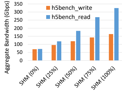
Figure 19: Aggr. bandwidth for h5bench I/O in case-2 (4 nodes).
