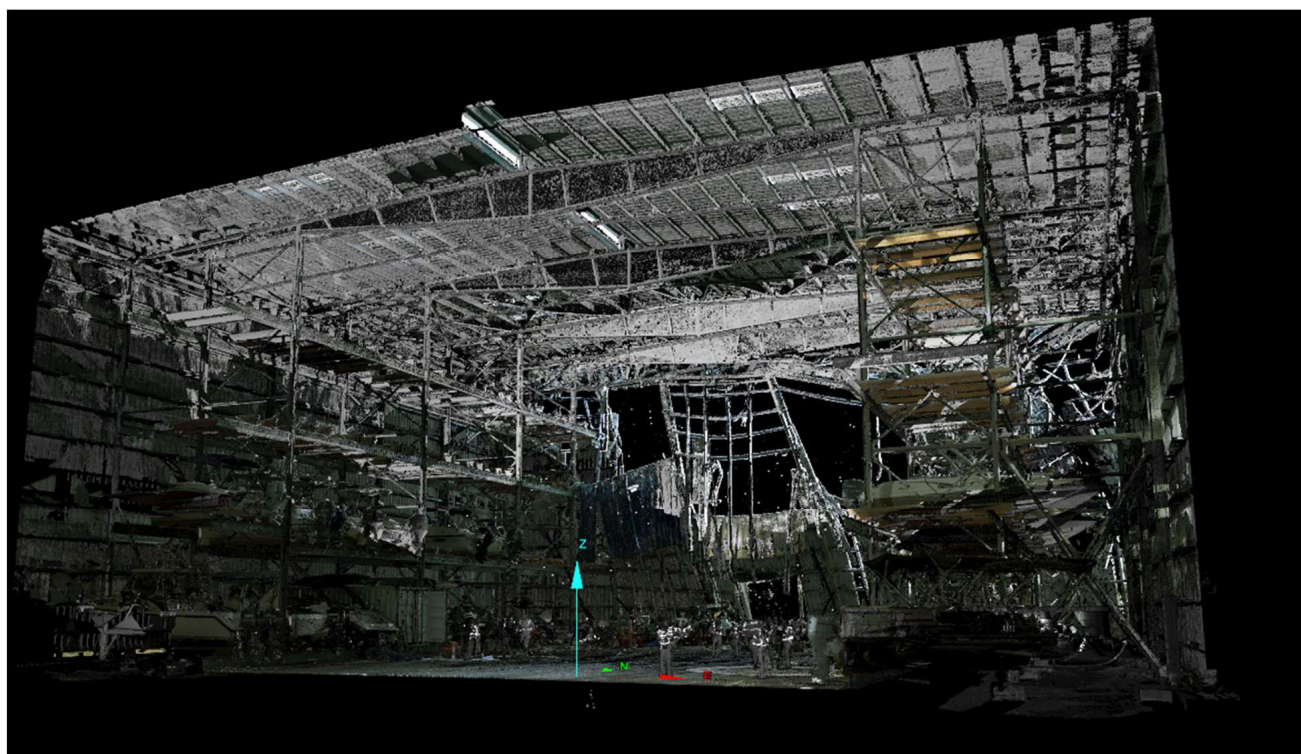
FIGURE 6 | 3D point cloud from lidar scans of the interior of the damaged marine storage building before cleaning (removal of debris to expose the structural system).
