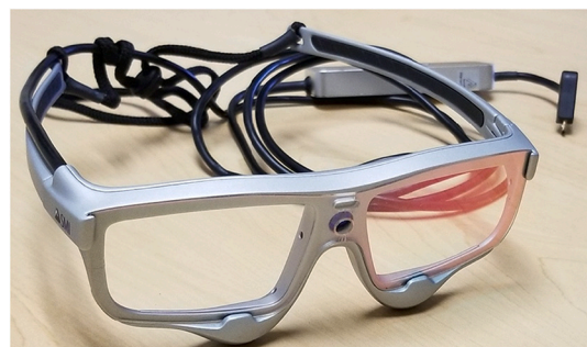
Fig. 1. A typical pair of eye tracking glasses (SMI Eye Tracking Glasses 2.0).
