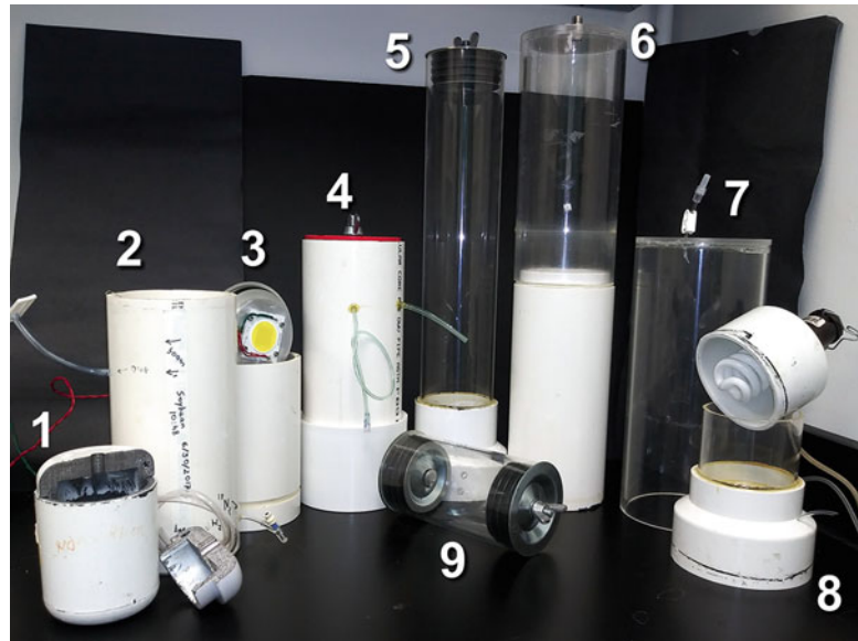
Fig. 4 Examples of labeling chambers: (1) A lead pig container (1/2" thick) with split lid for labeled root (see also Fig. 2); (2) A pot with a gas inlet (top) and an outlet for water supply and/or drain for labeling roots with radioactive gas; (3) An opaque whole-plant gas labeling chamber with built-in LED light on top; (4) An opaque whole-plant gas labeling chamber with gas inlet and outlet; (5–7) A variety of transparent whole-plant gas labeling chambers, 4–6 inches in diameter; (8) Plant labeling chamber with fluorescent light; (9) Labeling container for small plants
