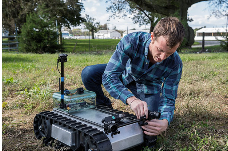
Fig. 1 Adjusting cameras on a modified SuperDroid LT2 Tracked ATR platform. For simplicity, the design described in this method includes a single camera sensor, but it is easy to add more sensing capabilities. Pictured here are additional sensors, including one extra RGB camera, an RGBD camera, analog video transmission, GPS, and external waterproof electronics housing. Camera rails allow quick and easy outfitting of the robot for various phenotyping experiments
