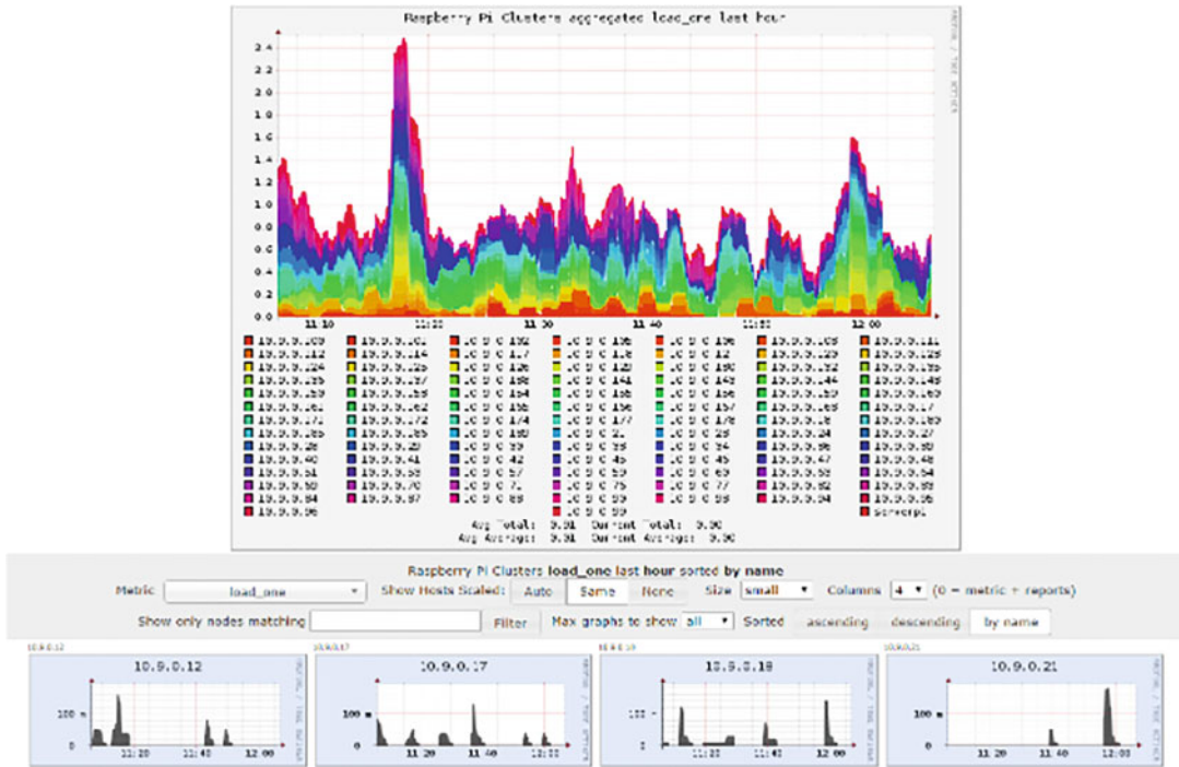
Fig. 5 Ganglia interface showing CPU load of each Pi in the bramble. CPU load for four camera systems are individually highlighted in bottom panels
