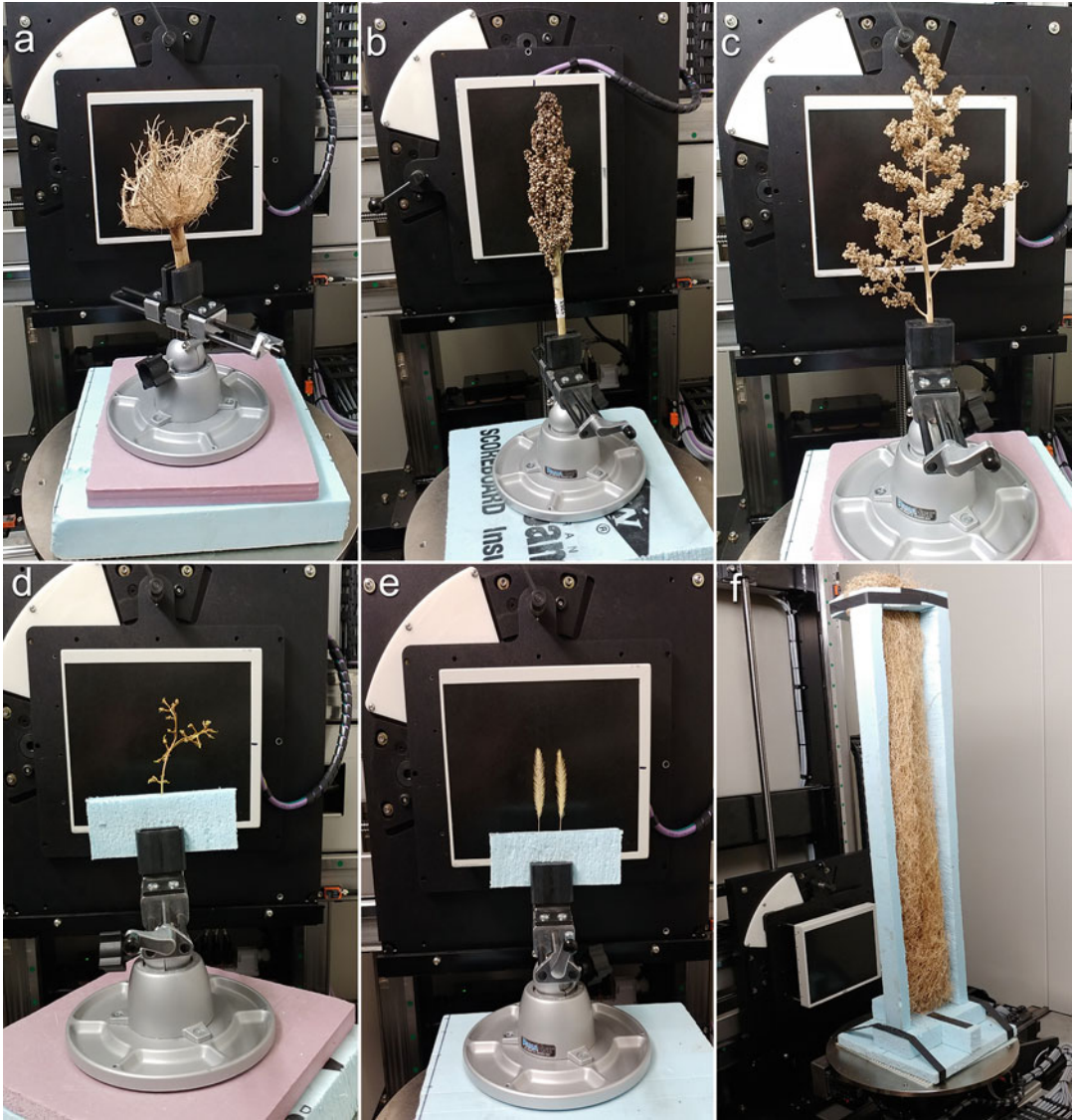
Fig. 1 Various fixtures for securely holding samples during rotation while scanning; the detector in each image is 20 \times 24 cm for scale. (a–c) A portable vise is used to directly clamp a maize root crown (a) , and panicles of sorghum (b) and quinoa (c) in front of the detector for scanning. (d, e) Rectangular pieces of expanded polystyrene (EPS) are used to hold thinner samples like grape rachis (d) and Setaria panicles (e) in the clamp during scanning. (f) An excavated switchgrass root system is secured within a frame cut from a single EPS board and mounted directly to the instrument turntable
