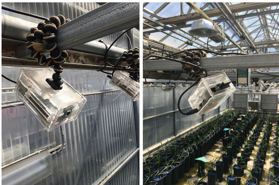
Fig. 2 Raspberry Pi camera setup (case, WiPi dongle, power cord) from two views attached to scaffold with a flexible tripod
