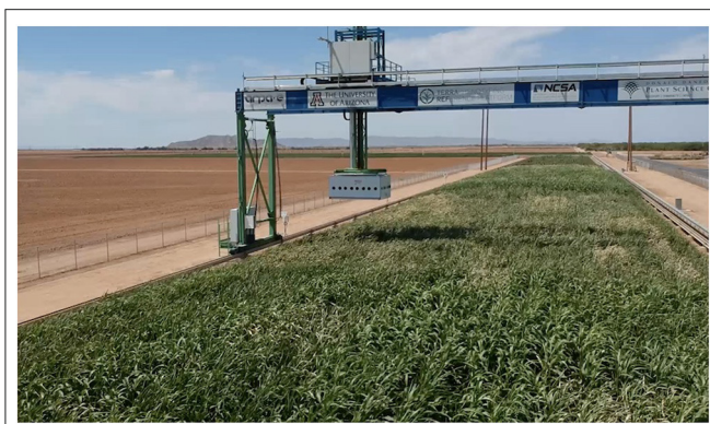
FIGURE 2 | The TERRA-REF Field and Gantry-based Field Scanner in Maricopa, Arizona, with sorghum being grown in the field.
