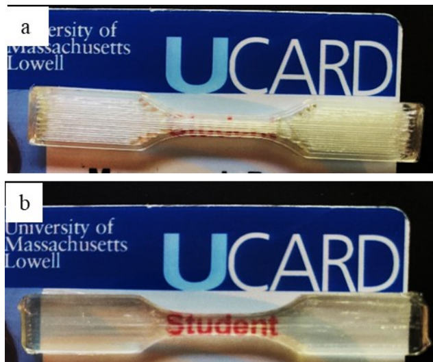
Figure 5. Effect of extruder temperature on transparency of samples printed at a. 180 °C (sample condition A); b. 220 °C (sample condition J).
