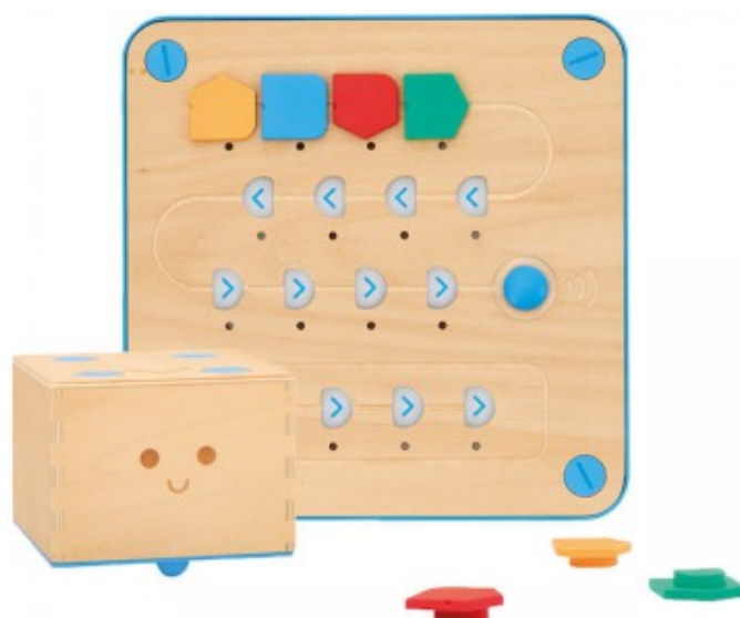
Figure 2. Cubetto toy robot with programming board and tiles. Produced by Primo Toys.
