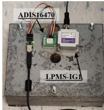
Figure 2. Experimental setup used for characterizing the IMUs' noise floor.
