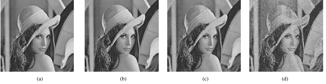
Fig. 11: Received Lena pictures of URadio-rGO-D4G50 using 16-QAM with different distances between Alice and Bob: (a) distance = 90 cm, SNR = 18.8 dB; (b) distance = 100 cm, SNR = 15.4 dB; (c) distance = 120 cm, SNR = 10.86 dB; (d) distance = 150 cm, SNR = 3.9 dB.
