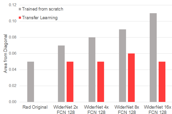
Figure 5. Area from the diagonal of reliability plots with and without transfer learning (TF). TF prevents this error metric from increasing as the model capacity increases. Best in color.
