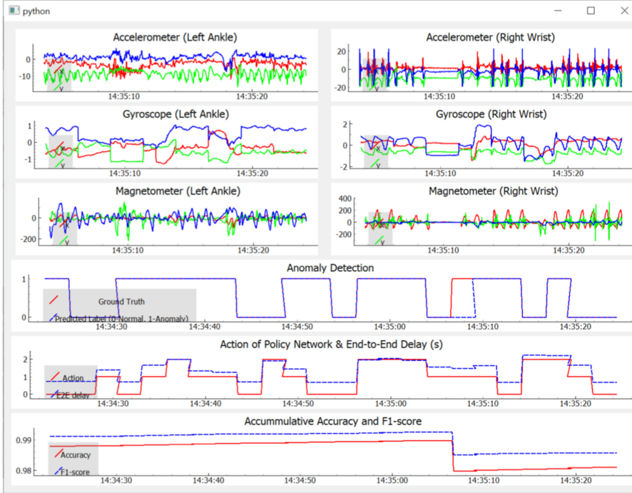
(b) Result panel: raw sensory signals, AD performance and associated actions.
