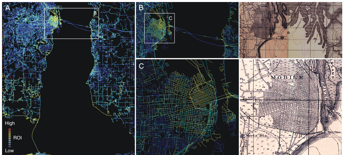
Fig. 10. Maps of the road overlap indicator (ROI) metric for the Mobile Bay (Alabama) study area in 1920, (a) shown for the whole study area, and (b)-(c) shown for the city of Mobile, at different levels of detail, including the underlying historical map. Shown is the ROI for each road segment, indicating whether a road likely existed in the year the historical map was created (light blue, yellow), dark blue roads likely did not exist yet. (For interpretation of the references to color in this figure legend, the reader is referred to the web version of this article.)
