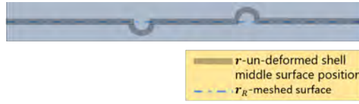
Fig. 3: The schematic of level set representation of a modified shell model
