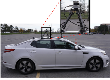
Figure 7: The Ouster OS1-64 LiDAR mounted on a vehicle.
