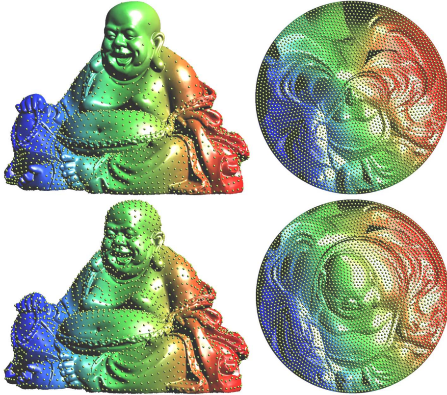
Figure 13. Different encoding mappings from the manifold to the planar disk.
