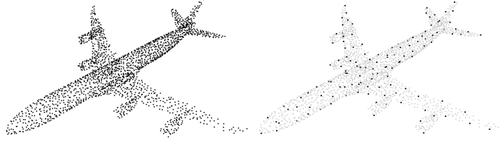
Figure 6: Farthest point sampling (left:origin cloud, 2048 points; right:after sampling, 128 points))
