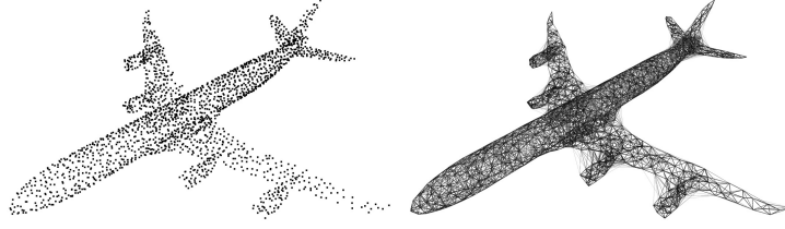
Figure 14: Unordered point cloud (left) and undirected weighted graph constructed by Delaunay Triangulation method (right)
