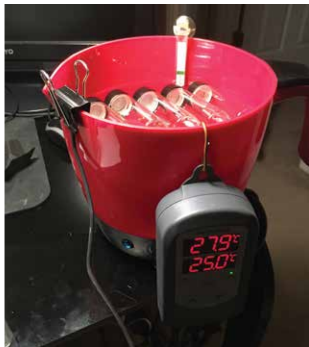
Fig. 2. Quantifying the effect of thermal tolerance on pollinator foraging behavior. Students collected bee and fly visitors of plants near their homes and either used their kitchens or desks to operate the water baths used as devices to quantify critical thermal maxima in pollinators. Photo credit: Alonso Delgado
