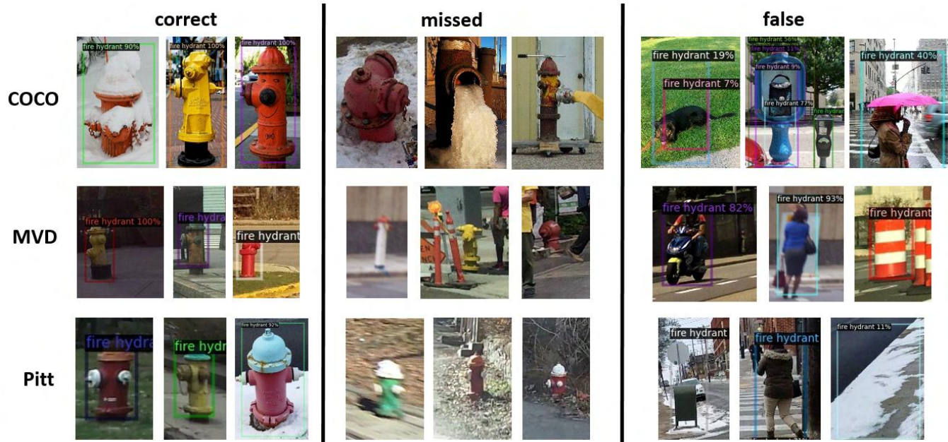
Fig. 8: Qualitative results from fire hydrant predictions: CARLA-trained model tested on all three data sets. Shown are correct, missed and false detections.
