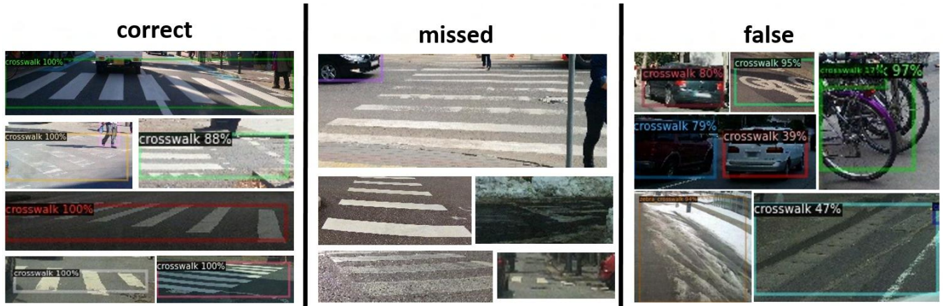
Fig. 4: Qualitative results from crosswalk predictions: CARLA trained model tested on MVD dataset. Shown are correct, missed and false detections.
