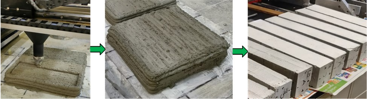
Figure 3: The 3D printed slab: (a) while printing, (b) after printing, and (c) after cutting into desired dimensions for testing.
