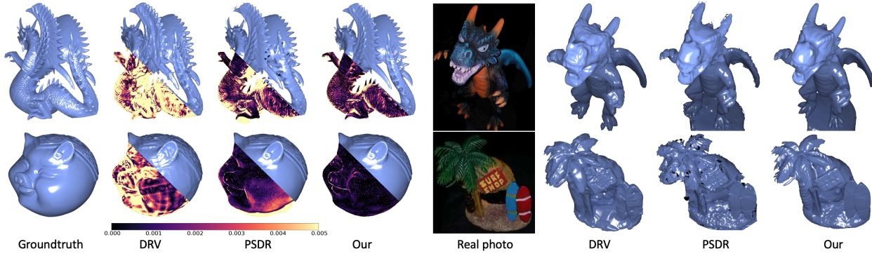
Figure 6. Comparison of recovered geometry on synthetic ( left ) and real data ( right ) with baselines DRV [4] and PSDR [21]. On synthetic data, we achieve the highest geometric reconstruction accuracy among the inverse rendering methods designed for flashlight photography. For real data, we show a captured photo for reference due to lack of ground truth geometry.
