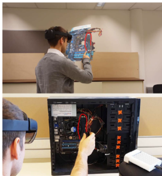
Figure 1: Top: Remote expert view, including annotations. Bottom: Local operator’s view. The expert is adding annotations which are visible to local operator.
