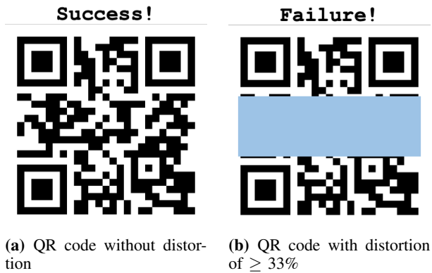
Fig. 1: Example of a successful and failed QR code scanning.
