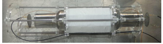
FIG. 2. NaI-033 crystal detector module. The crystal is wrapped with ten layers of PTFE tape and coupled to two Hamamatsu R11065 PMTs via optical grease. The assembly is held in place by acrylic holders, nylon nuts, and three stainless-steel threaded rods.
