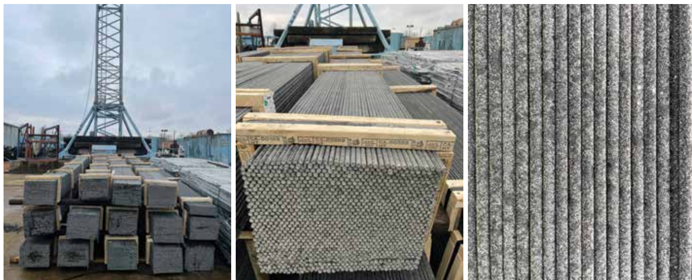
Fig. 1: BFRP bars used to reinforce topping slabs
