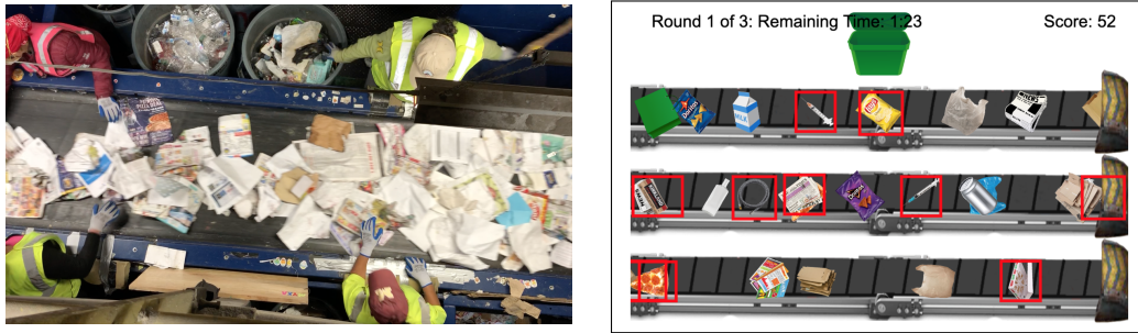
Fig. 1. Left: Conveyor belts for trash sorting at a real Materials Recovery Facility (MRF). Right: The Simulated MRF that we developed and deployed for our experiments. Some objects are highlighted with a box that is generated by a Machine Learning Assistant (MLA) to help the worker to recognize objects that need to be removed from the conveyor belts.
