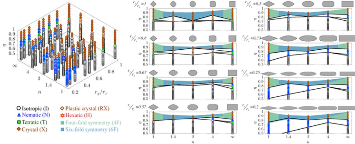
**Fig. 8.** Phase diagram for hard superellipses as a function of the aspect ratio ( $r_y/r_x$ ), particle shape parameter ( $n$ ), and area fraction ( $\eta$ ). Phases indicated as: (O) isotropic, ( $\Delta$ ) nematic, ( $\blacksquare$ ) tetratic, ( $\diamond$ ) plastic crystal, or ( $\blacklozenge$ ) crystal, with symmetry indicated as ( $\blacksquare$ ) four-fold or ( $\blacksquare$ ) six-fold. Hexatic phase ( $\star$ ) from large system size literature results.<sup>11,12</sup>
