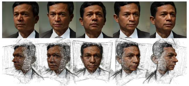
Figure 2. COLMAP [32, 33] reconstruction of 128 frames of synthesized video (top) which followed an oval trajectory. The resulting dense, well-defined point cloud (bottom) is indicative of highly multi-view-consistent rendering.
