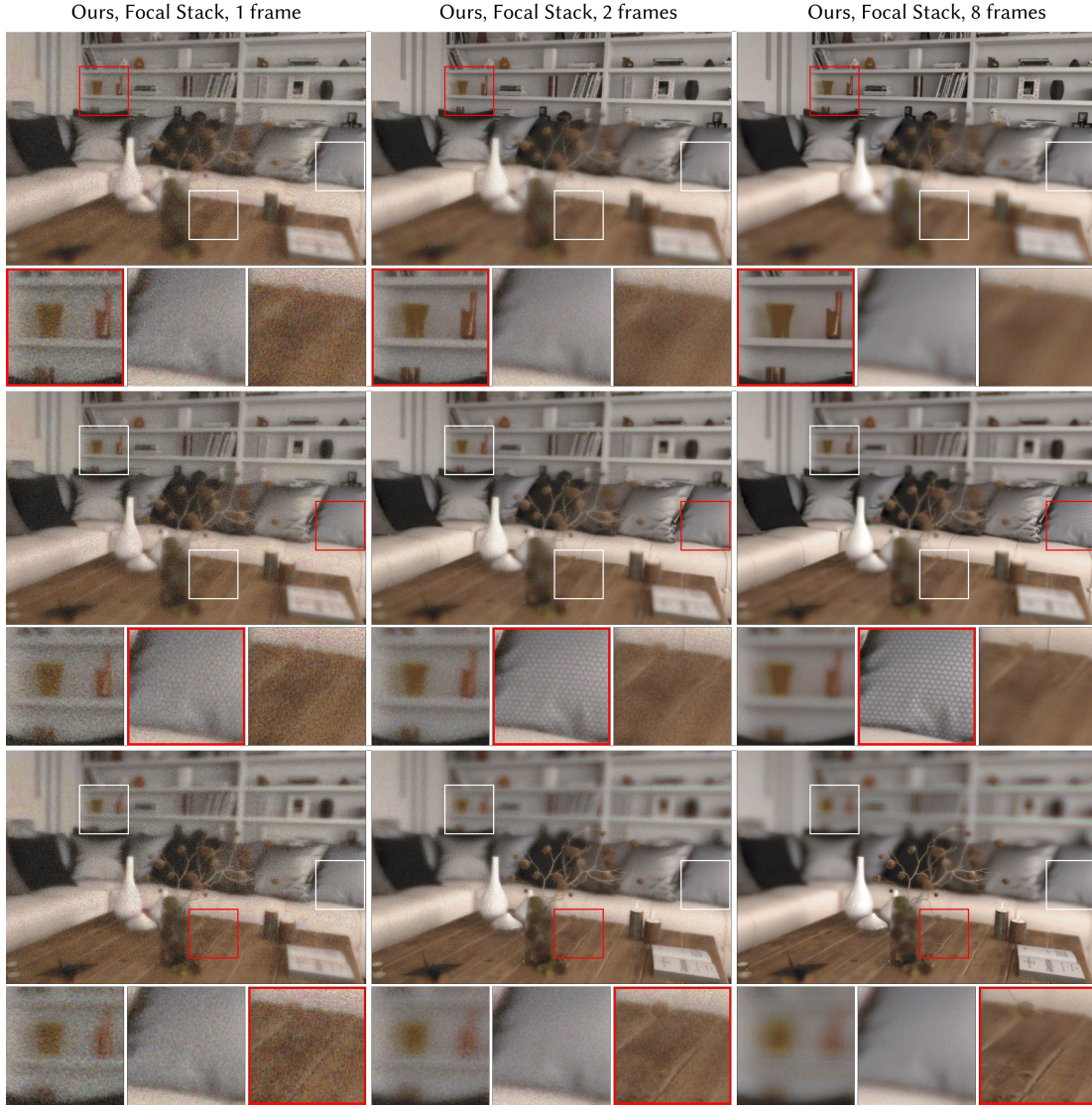
Fig. S4. Simulated evaluation of focal stack supervision with 1, 2, and 8 frames from left to right on ideal continuous SLMs. Focused regions are highlighted with red boxes, that from top to bottom, indicate far, center, and near distances. Even without quantization on an ideal SLM, the supervision with only 1 or 2 frames is overconstrained by the focal stack and cannot fully reproduce the desired natural defocus blur.
