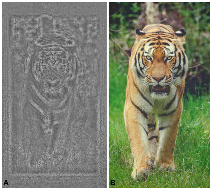
Fig. 4. Experimentally captured 2D holographic image and corresponding phase pattern. We present the holographic image (B) obtained using SLED along with the SLM phase pattern (A) that was automatically optimized using the proposed CITL strategy. This result shows sharp image details without noticeable speckle artifacts. Image Credit: Eirikur Agustsson and Radu Timofte, ETH Zurich.
