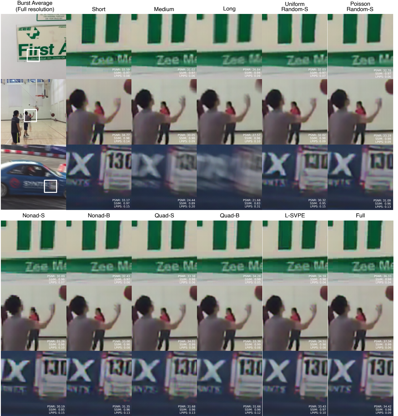
Fig. C1. Qualitative comparison of baselines. Each row of individual images (carried over to create two larger rows) shows an example frame of the average of all the video segment frames ( Burst Average ) at full resolution and a 100 \times 100 crop of a region for all baselines. Row 1: An example of a little to no motion scene. The lettering is most clearly recovered and free of color artifacts with L-SVPE and Full . Row 2: An example of a scene with local motion. The reconstruction of the man's hand and the deburring of the basketball is best observed in spatially varying coded exposures. L-SVPE is also relatively free of color artifacts. Row 3: An example of a scene with global motion. The "X" on the side of the car and the lines on the logo next to it are clearly recovered by L-SVPE while methods like Short and Quad introduce more blurring artifacts.
