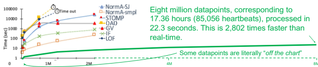
Figure 13: (Most of this figure is taken from [3], only the green elements are new). The scalability of various algorithms on increasing large subsets of a long ECG trace. All algorithms except DAMP are limited the first 2M data points by [3]. Note that the Y-axis is logarithmic.
