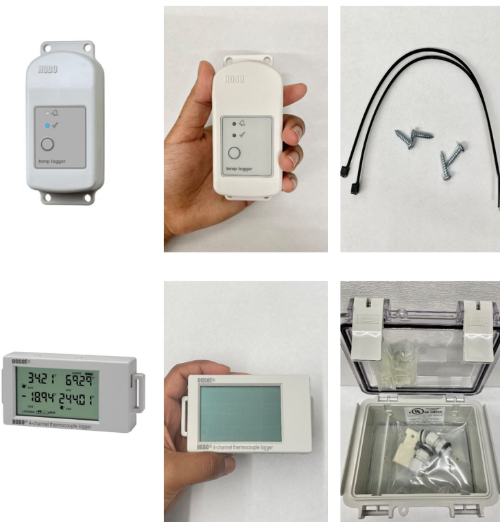
Figure 3: (Top panel) The HOBOMX2300 Wireless Temperature Data Logger and cable ties/screws for mounting. (Bottom panel) The HOBUX120 4-Channel Thermocouple Logger and Thermocouple case and screws for mounting.
