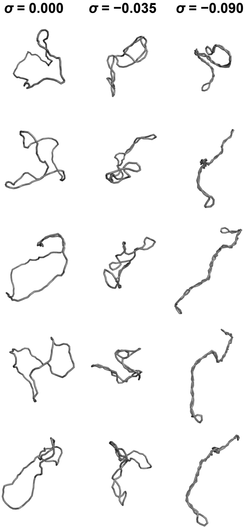
Figure S2: Randomly-chosen plasmid structures from our main simulation ( L_{\text{circle}} = 2,686 bp, 100 beads, l_{\text{HC}} = 2 nm) at three superhelical densities . Comparing structures from the center column to those in the right column, we see that plectonemic end loops become tighter and plectonemic stems become straighter as \sigma goes from -0.035 to -0.090 .
