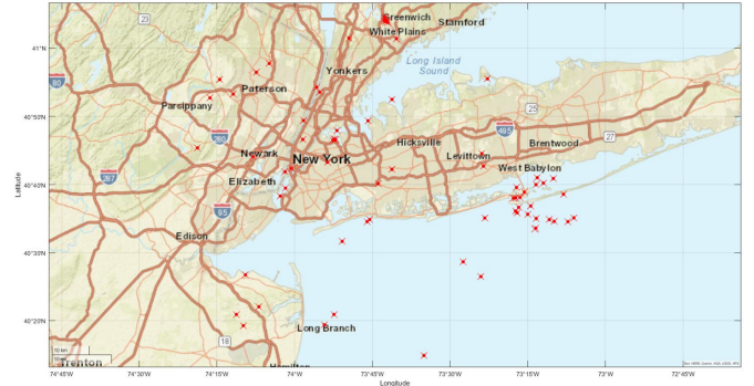
Fig. 2. Example of aircraft positions in the received ADS-B messages
