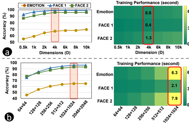
Figure 5: (a) Impact of dimensionality on HDFace accuracy & training performance. (b) Impact of DNN configuration on classification accuracy and training performance.
