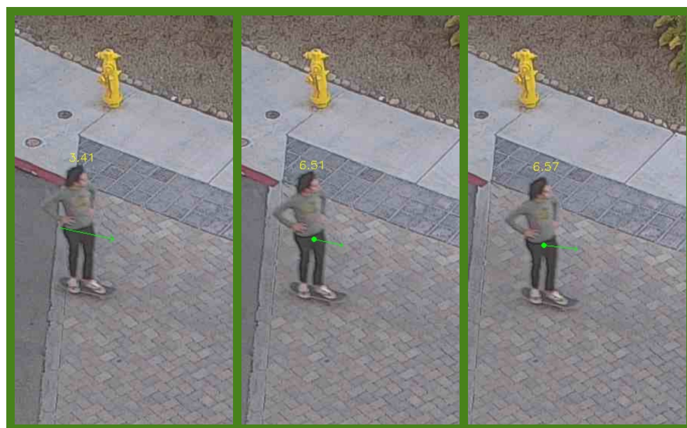
Figure 36. First-order average object velocity estimation to predict time to collision (TTC). Units of numbers shown in yellow are pixels/frame.
