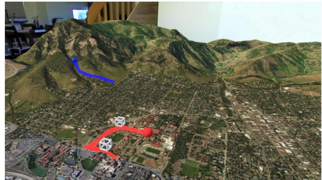
Figure 2: Trajectories (lines) and current GPS positions (spheres) of the human field team (blue) and the field robot (red). White cubes represent robot-collected 3D reconstructions that users can select to view and manipulate the corresponding MR dense point clouds above the 3D terrain table.
